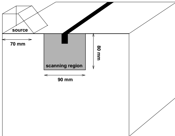
Figure 7. Experimental configuration, where the source is perpendicular to a single groove on the top of the block, while the detector scans the side.
