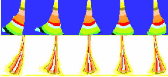
Figure 4: Traveltime tables for five Gaussian beams all shot from the same surface location with different takeoff angles. The top panel shows the real part of the traveltime, and the bottom panel shows the exponential of the imaginary part of the traveltime at a reference frequency. The real part of the traveltime has moderate curvature, and the imaginary part of the traveltime causes exponential decay of energy away from the raypath.
